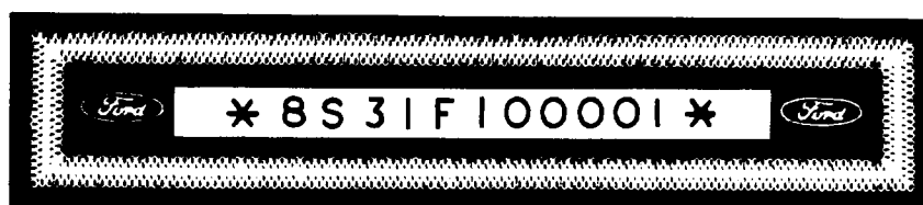
FIG. 2—Typical Vehicle Identification Number (VIN) Tab—Fairlane Shown
